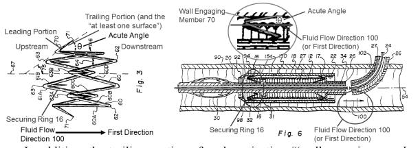
In addition, the trailing portion of each projection ("wall engaging member 70") comprises at least one surface that is preferentially oriented to extend at an acute angle to a first direction ("fluid flow direction 100"). *See* annotated Figs. 3 and 6 of Lazarus above; *see also* Exh. 1005, 5:47-51.
