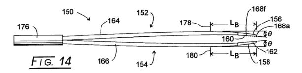
Figure 14 is a plan view of the forceps according to Eggers '142. Ex. 1007, 5:3–5, 5:11–12. The only difference between this embodiment and the one illustrated in Figures 8–11 is that the former has insulative spacers on one grasping surface, while the latter has insulative spacers on both grasping surfaces. *Id.* at 9:34–36, 11:49–51, 13:22–23; *compare id.* at Figs. 8, 9, *with id.* at Figs. 12, 13.
