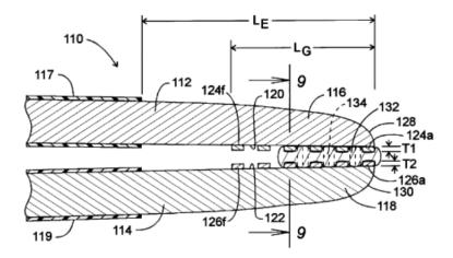
Figure 8 is a partial sectional view of an embodiment of forceps according to Eggers '142. Ex. 1007, 4:61–62. It shows strips 124a–124f having a uniform thickness T1, and 126a–126f having a thickness T2. *Id.* at 9:40–41, 9:49–50. The strips "are aligned for movement into mutual contact when in a closed orientation." Ex. 1007, 9:66–10:1.
