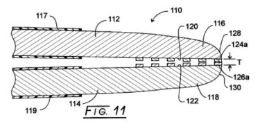
Figure 11 shows "strips or insulated regions 124a and 126a having been moved into mutual contacting relationship." *Id.* at 10:47–49. According to Eggers '142, "[u]pon further pressure being made by the user,
