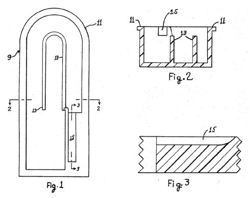
Figure 1 is a top view, and Figures 2 and 3 are cross-sectional views, of catheterization tray 9. *See id.* at col. 2, ll. 21–29. Lubrication channel 15
