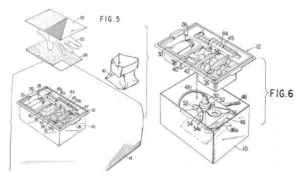
Figures 5 and 6 depict box 10, on the open top of which is mounted tray 12, enclosed within wrap 14. *Id.* at col. 1, ll. 60–62. The entire assembly is enclosed within envelope 16. *Id.* at col. 1, ll. 62–63. Serany describes that the wrap serves as a sterile field when removed from around the box and flattened thereunder. *Id.* at col. 2, ll. 17–20.
