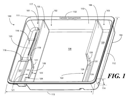
As shown in Figure 1 above, tray 100 has first compartment 101 for accommodating syringes and second compartment 102 for accommodating the catheter assembly. *Id.* at col. 5, ll. 17–20. The '190 patent explains that
