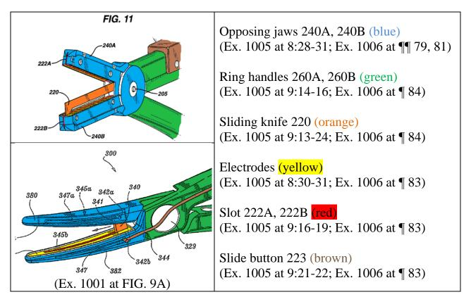
Applicant notes that while *Witt* actually illustrates a slide button 223, the '536 Patent neither illustrates nor describes the device to actuate the knife of Fig. 9A.
