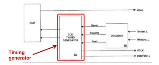
(Ex. 1107, King at Fig. 2 (annotated) and 5:51-58.) The CCD Timing Generator 42 generates a "sequence of vertical and horizontal clock cycles required to completely transfer the image residing in the readout cells to the Camera Control Unit (CCU) 36." (Ex. 1107, King at 8:4-7.) Thus, King's CCD Timing Generator 42 is a "timing generator, for generating a timing signal particular to said camera head, wherein the timing signal actuates said imager," as required by claim 2.
