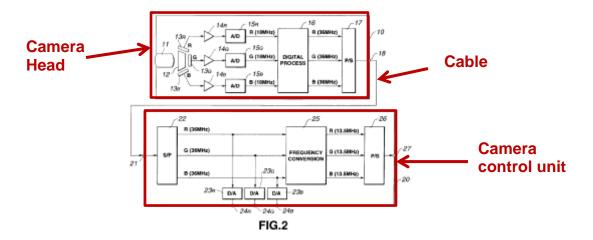
(Ex. 1108, Nakamura at Fig. 2 (annotated); *see also* Nakamura at 1:8-10 ("This invention relates to a method and apparatus for transmitting digital video signals obtained on imaging by a CCD imaging device."), 4:25-26; Ex. 1109, Grindon Decl. at ¶ 109.)
