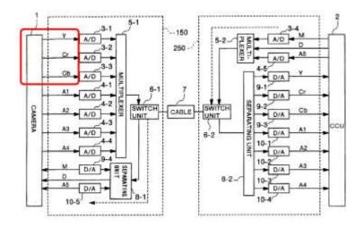
(Ex. 1103, Eto at Fig. 1 (annotated).) Further, Eto states that this imager is for generating a stream of video data. It states that "a video (picture) signal obtained from a <u>television camera 1 is three sorts of video signals</u>, i.e., a luminance signal 'Y' and two sorts color difference signals 'Cr' and 'Cb' instead of the respective video signals R, G, B." (Ex. 1103, Eto at 7:7-19 (emphasis added).) (*See also* Ex. 1109, Grindon Decl. at ¶ 52.)
