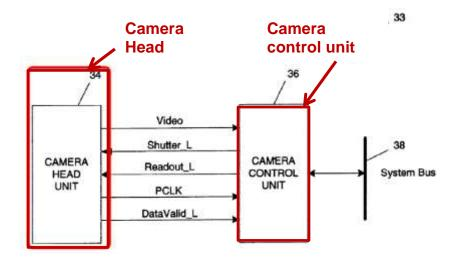
(Ex. 1107, King at Fig. 1 (annotated).) The camera head includes a CCD image sensor and a CCD timing generator (42):
