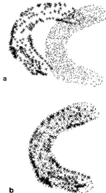
Fig. 8. Registration of the 3D points acquired by the pointer with the splint surface segmented on CT images. (a) Initial position. (b) Final position.
