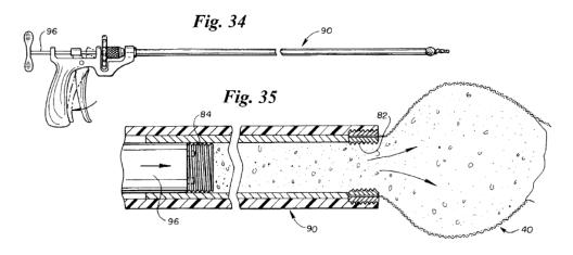
Figure 34 depicts using the gun-like device to fill the bag, and Figure 35 depicts a cross-section of the end of the device. *Id.* at 5:30–32. As shown in Figure 35, the bag includes a threaded fill port with internal threads 82 to receive threaded screw 84. *Id.* at 10:20–22. Plunger 96 pushes screw 84 along with the graft material towards bag 40 and, at the end of the stroke, turns the screw to seal the bag. *Id.* at 10:31–34.
