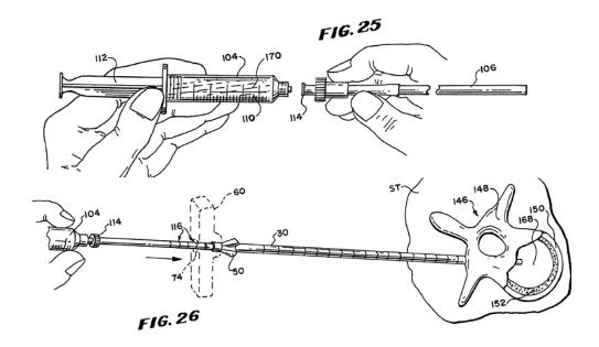
Figure 25 is a perspective view of conventional syringe 104 being joined to injection nozzle 106, and Figure 26 is a perspective view showing the nozzle being deployed through cannula instrument 30 such that the nozzle extends a selected distance beyond the distal end of the cannula instrument and into cavity 168 of vertebral body 148. *Id.* at 4:41–47, 10:32–33, 16:1–9.
