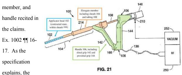
handle is used to expand the applicator head once it has been inserted into the uterus, enabling ablation treatment. Ex. 1001 at 11:61-67 ("[T]he applicator head is slidably disposed within the sheath (FIG. 21) during insertion of the device into the uterine cavity, and the handle 106 is subsequently manipulated to cause the applicator head 102 to extend from the distal end of the sheath 104 (FIG. 22) and
