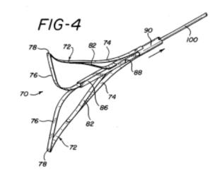
the actuator tube 90." *Id.* Ortiz explains that "when actuator tube 90 is retracted, i.e., moved proximally relative to the support shaft 100, the fingers 72 are spread apart and the platform 70 is expanded into a tulip-shaped configuration." *Id.* at 5:28-31, FIG. 4 (shown here); *see also* Ex. 1002 ¶ 35.
