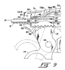
rack tube or sleeve 36." Ex. 1006 at 6:31-34; FIG. 9 (shown here). As Dr. Pearce explains, and as discussed in further detail with respect to limitation 1.4, the gear rack tube 36 teaches or suggests the claimed frame. Ex.  $1002 \, \P \, 97$ .
