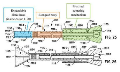
elongate body, and a distal actuating mechanism (*i.e.*, a handle). *Id.* at FIGS 25 (head collapsed), 26 (head expanded); Ex. 1002 ¶ 32. The device described in Yoon "can be made of an
