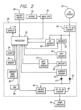
Figure 2 depicts a block diagram of power management system 28, which includes processor 42, battery 26, voltage sensor 49, and current sensor 50. *Id.* at 3:41–42, 4:54–58. Remaining battery life is determined "based on the amount of charge remaining in the battery and the present current draw from the battery" and is depicted on a display in fifteen minute increments. *Id.* at 2:4–5, 7:15–27, 10:38–42, Fig. 3. Additionally, audible
