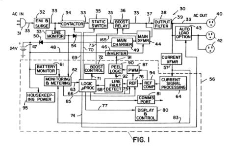
Figure 1 presents a block diagram of uninterruptable power system 30, connected between an AC power source (at inlet plug 31) and a critical load, e.g., a computer (at output terminal 40). *Id.* at 4:56–59, 4:64–67, 5:2–6. Power system 30 includes inverter 46 and battery 47. "When power from the AC power mains fails, an inverter 46 is turned on, and DC power is supplied to the inverter from an auxiliary power supply battery 47 on a DC bus 48." *Id.* at 5:20–23.
