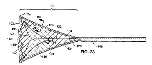
Figure 23 depicts the applicator head of the ablation device of the second embodiment. *Id.* at 3:55–56. The '989 patent states:
