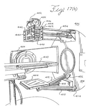
Specifically, Figure 17(b) above shows wall-mounted cone beam computerized tomography system 400 includes an x-ray source, such as x-ray tube 402, and flat-panel imager 404 mounted on gantry 406. *Id.* at 19:41–43. X-ray tube 402 generates beam of x-rays 407 in a form of a cone
