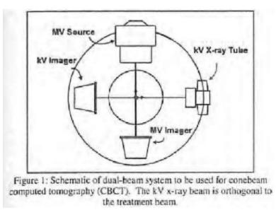
*Id.* at 5. As shown in Figure 1, "[t]wo fluoroscopic imaging systems are attached to a Philips SL-20 medical linear accelerator; one detects the megavoltage image, the other a kV image produced with a kV beam projected at 90° to the treatment beam axis." *Id.* at 4. Jaffray 1997 states that the "gantry is rotated continuously" in order to generate a "conebeam imaging sequence consist[ing] of ~100 exposures over 194° of rotation." *Id.* at 5 (alteration in original).
