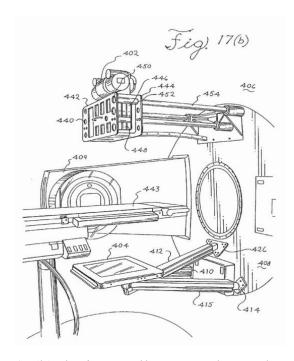
Specifically, Figure 17(b) depicts wall-mounted cone beam computerized tomography system 400 including an x-ray source, such as x-ray tube 402, and flat-panel imager 404 mounted on gantry 406. Ex. 1101, 19:64–20:2. X-ray tube 402 generates a beam of x-rays 407 in a form of a cone or pyramid. Ex. 1101, 20:2–4. Flat-panel imager 404 employs amorphous silicon detectors. Ex. 1101, 20:6–7.
