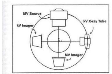
Figure 1: Schematic of dual-beam system to be used for conebeam computed tomography (CBCT). The kV x-ray beam is orthogonal to the treatment beam.
