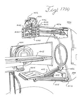
Specifically, Figure 17(b) depicts wall-mounted cone beam computerized tomography system 400 includes an x-ray source, such as x-ray tube 402, and flat-panel imager 404 mounted on gantry 406. Ex. 1201, 19:64–67. X-ray tube 402 generates beam of x-rays 407 in a form of a cone or pyramid. Ex. 1201, 19:67–20:2. Flat-panel imager 404 employs amorphous silicon detectors. Ex. 1201, 20:6–7.
