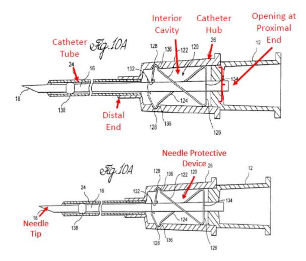
According to Petitioner, and as shown in Figure 10A, Woehr discloses a "catheter insertion device" comprising the claimed "catheter hub" 26, "needle" 16, and "needle protection device" 120. *Id.* at 12–14, 23–24.
