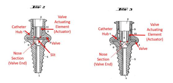
According to Petitioner, and as shown in the above Figures 2 and 3, Tauschinski discloses valve actuating element 10 with a nose section having a tapered end, slidingly disposed in catheter hub 1, and configured to actuate valve 3 to open slit 8. *Id.* at 19 (citing Ex. 1004, 3:21–36).
