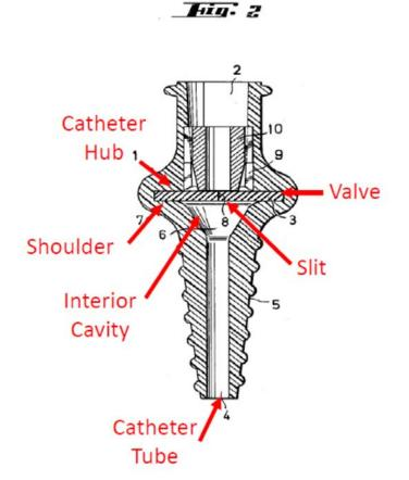
As shown in Figure 2, Petitioner asserts that Tauschinski discloses valve 3 with slit 8 configured to obstruct fluid flow through catheter hub 1. *Id.* at 16 (citing in-part Ex. 1004, 2:7–19). Petitioner reasons that it would have been obvious to modify Woehr "by adding protective elements, such as a valve to prevent the emergence of blood," as disclosed by Tauschinski. *Id.* at 17–18 (citing in-part Ex. 1002 ¶ 73).
