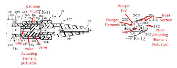
According to Petitioner, Figure 11 (above-left) depicts valve actuating element 220, and as shown in Figure 12 (above-right), valve actuating element 220 has two plunger elements and gap 306 "therebetween . . . that permits fluid to flow therethrough." Pet. 21 (citing: Ex. 1005, 7:29–36; Ex. 1002 ¶ 79).
