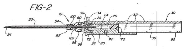
Figure 2 depicts a cross-sectional view of Van Heugten's catheter assembly 10. *Id.* at 2:6–10, 19–21. In particular, Figure 2 illustrates catheter assembly 10 with catheter 50 and needle 24, which needle guard 30 covers upon retraction of needle 24 to prevent inadvertent needle injury to the user or others. *See id.* at 2:36–39, 3:34–58. Catheter assembly 10 also includes valve membrane 110, which is illustrated in Figures 4a and 4b, which we also reproduce, below:
