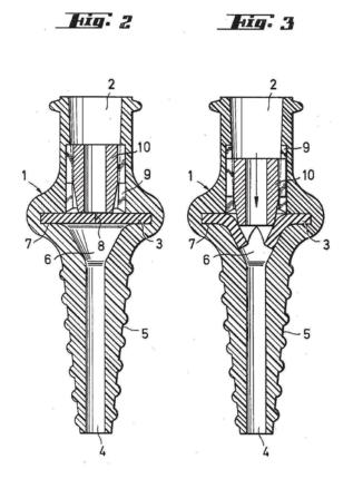
According to Tauschinski, Figures 2 and 3 depict a connector with a slit sealing disc. *See id.* at 2:62–68. In particular, these figures depict member 10 slidable within hollow-conical portion 2 and disc 3 provided with central slit 8. *See id.* at 3:17–25. Figure 2 depicts disc 3 as closed, with Figure 3 depicting member 10 advanced downward and within slit 8 of disc 3 to open the slit. *See id.* at 3:29–36.
