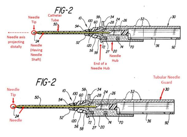
According to Petitioner, and as shown above, Figure 2 depicts Van Heugten's "catheter hub" 52, "needle" 24, and "needle protective device" 30. *Id.* at 38, 39, 45.
