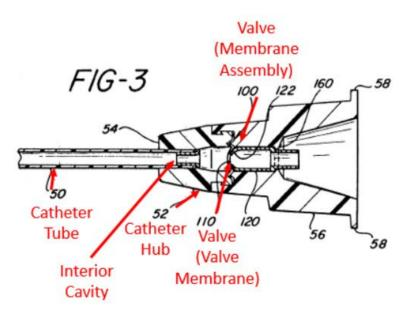
According to Petitioner, and as shown in Figure 3, Van Heugten also discloses the claimed "valve" 100, 110. *See* Pet. 40–42 ("a POSA would have understood Van Heugten to disclose the valve membrane 110 having one or more slits") (citing Ex. 1002 ¶ 134).
