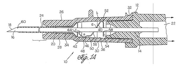
Woehr describes Figure 1A as depicting catheter 10 including needle hub 12, needle 16 with needle tip 18, catheter hub 26, and needle guard 40 in the form of a unitary spring clip. *Id.* at 4:8–28, 50–51. As needle 16 is withdrawn from a patient, needle guard 40 "automatically snaps into a retracted position" to block needle tip 18 to prevent accidental contact to the health care practitioner. *Id.* at 4:43–49.
