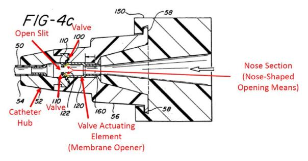
According to Petitioner, Figure 4c depicts "valve actuating element" 120 comprising a nose section with a tapered end 122. *Id.* at 43–44 (citing Ex. 1006, 4:31–36, 4:43–49).
