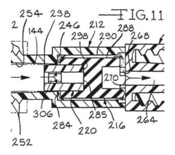
The portion of Figure 11 depicts the assembly in an open position. *See* Ex. 1005, 8:41–43. As shown in Figure 11, and denoted by arrows, when Arnett's actuator 220 presses against septum 216, a seal between shoulder surface 284 and septum shoulder 246 breaks, thus allowing fluid to flow *through fluid passageway 306 and through fluid passageways 290. See id.* ("fluid is free to flow from the luer 140 through the fluid passageway 306 of the actuator 220 to the chamber fluid passageways 290").
