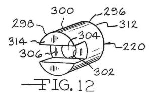
As described by Arnett, Figure 12 depicts actuator 220 including septum contact surface 312, an opposed fitting contact surface 314, and fluid passageway 306. *Id.* at 7:29–39. As discussed above in connection with Figure 11, *fluid passageway 306 allows fluid to flow around septum 216 and through fluid passageways 290. See id.* at Fig. 11, 8:41–44.
