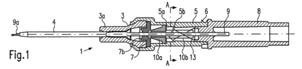
Woehr describes Figure 1 as depicting its catheter insertion device 1 in a ready-to-use position. *Id.* at 1, 2. Device 1 comprises distal hub 3, catheter 4, hub element 5, and a check valve in the form of valve disk 7. *Id.* at 2. In the ready-to-use position, needle hub 8 is inserted into hub element 5, and hollow needle 9 extends through valve disk 7 and catheter 4, such that needle point 9a is exposed. *See id.* Valve actuating element 10 (shown as
