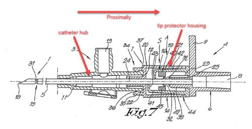
According to Petitioner, Figure 7 depicts Villa's "safety device" i.e. tip protector housing 20. *Id.* at 41. Petitioner asserts that "Villa discloses a 'protective device for a needle' that 'is intended to be used in combination with a catheter introducing needle . . . [and] discloses a hollow body or housing 20 that houses safety means 16 and blocking means 19." *Id.* at 41 (citing Ex. 1006 ¶¶ 1, 2, 47).
