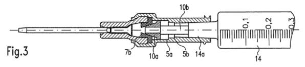
Woehr describes Figure 3 as depicting insertion of injection 14 into Woehr's catheter hub, with neck section 14a of injection 14a contacting plunger section 10b of valve actuating element 10. *Id.* at 3. Upon insertion of injection 14, cone-shaped contact section 10a of valve actuating element 10 presses against valve disk 7 to open the valve so that fluid may be supplied from injection 14 and into catheter 4. *Id.*
