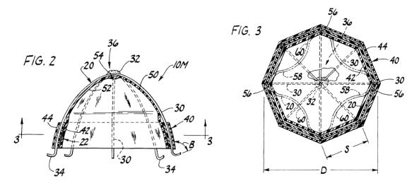
Figure 1 depicts "a vertical cross section of an artificial valve," and Figure 3 depicts "a cross section of the valve taken in the plane of line 3–3 of FIG. 2." *Id.* at 4:8–10. Artificial valve 10M shown in Figures 2 and 3 "is specifically configured for repairing a damaged mitral valve," although the '782 patent also discloses an artificial valve configured to repair a damaged pulmonary heart valve. *Id.* at 4:30–33.
