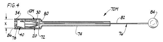
Figure 4 depicts "a vertical cross section of an instrument for implanting a valve using an endothoracoscopic procedure." *Id.* at 4:11–13. The instrument of Figure 4 includes tubular holder 72 and elongate tubular manipulator 74 attached to the holder for manipulating the holder into position. *Id.* at 7:34–36. The instrument further includes ejector 76 that is positioned in the hollow interior of holder 72 for ejecting an artificial heart valve from the holder. *Id.* at 7:36–39.
