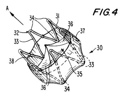
Figure 4 depicts artificial heart valve 30 having a generally cylindrical shape defined by stent member 32. *Id.* at 5:28–31. Stent member 32 is a wire formed into a closed zig-zag configuration having straight sections 33
