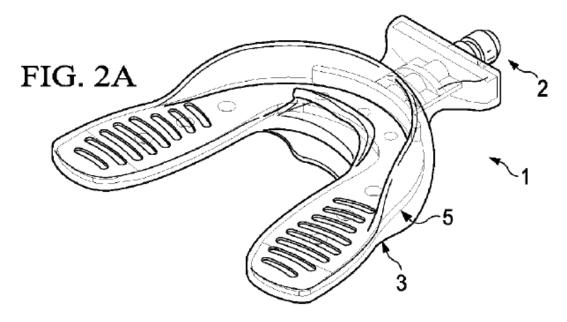
Figure 2A of the '184 patent, above, depicts bite plate 1 having connector 2 for attaching a motorized extraoral vibratory device (not shown). *See id.* at 7:53–54. The '184 patent explains that compared to conventional static force orthodontic devices "[a] faster method of orthodontic remodeling for a
