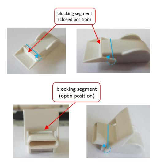
26. The vPEP® device includes a vane (red arrows below) configured to rotate the blocking segment between the closed position and the open position in response to the flow of air through the opening.
