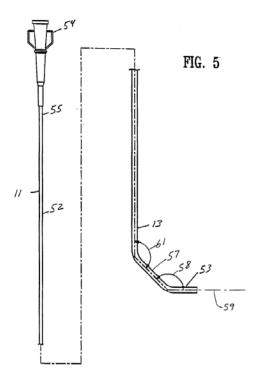
*Id.* at 17:1–15. Figure 5 illustrates outer catheter 11 comprised of main shaft section 52 and distal shaft section 13, with the latter comprised of first and second segments 53, 57 forming angles 58 and 61. *Id.* Angle 58 can be from about 90° to about 160°, and angle 61 can be from about 95° to about 165°. *Id.* at 17:6–11.
