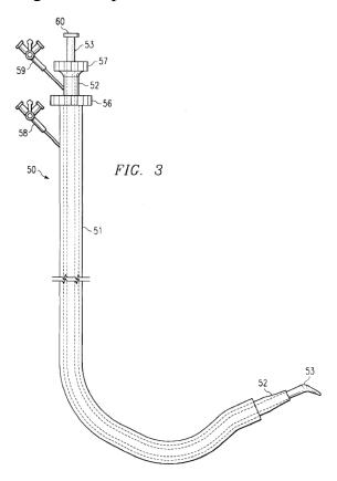
Figure 3 is a side view of triple catheter 50 comprising outer catheter 51, inner catheter 52, and obturator 53. *Id.* at 2:64–65, 4:63–5:3. Instead of "rely[ing] on specialized miniature adjustment mechanisms" such as screw 29 and cable 31 in Figures 1–2, "[t]he angle of outer guide 51 can be
