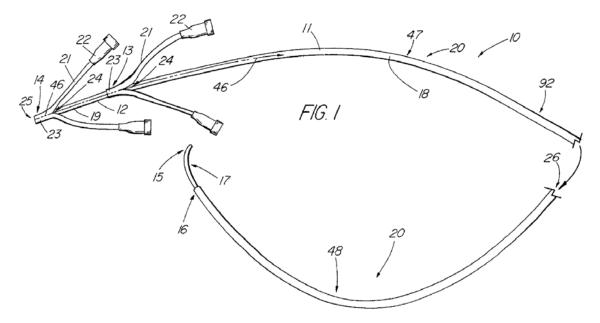
Figure 1 is a side view of introducer apparatus 10, which is composed of first introducer sheath 11 and second introducer sheath 12, with sheath 12 coaxially received within sheath 11. *Id.* at 4:8–9, 4:48–52, 5:20–23. Sheath 11 has preformed bend 20, comprised of proximal bend 47 and distal bend 48, that at least somewhat corresponds to the shape of a tortuous anatomical pathway to ease navigation of sheath 11 through the pathway to access the coronary sinus. *Id.* at 5:64–6:28, Figs. 3 & 3a.
