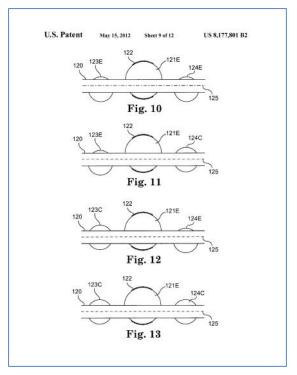
Accordingly, for many years prior to the effective filing date of the '853 patent, it was known that an eccentric abrasive element traces an orbital path having a larger diameter than the outer diameter of the rotational atherectomy device in the non-rotating state and the use of certain design features, such as placement and mass of stability elements on the drive shaft, can be used to control the orbital motion.
