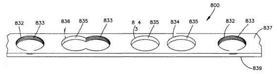
As described in Chan, Figure 8 illustrates bone plate 800 having "locking" holes 832 with threads 833 for engaging threads around the head of a locking bone screw, "non-locking" holes 834 with non-threaded or smooth inner surfaces 835, and "combination locking / non-locking" hole 836.
