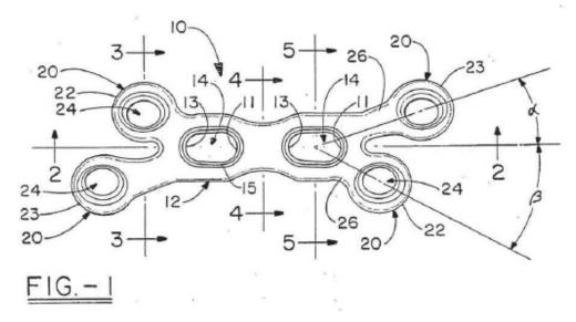
Figure 1 illustrates orthopedic plate 10 having a modified X-shaped profile, formed by central trunk portion 12 and two pairs of arms 20 extending diagonally from opposed terminal ends of central trunk portion 12. *Id.* at Abstract, ¶¶ 45, 47. In certain embodiments, plate 10
