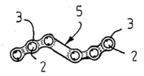
Figure 3 illustrates bone plate 5 having an S-shape, with screw holes 2 within screw rings 3. *Id.* at 2:18–22, 8:41–58. Screw holes 2 are "disposed at the ends of" plate 5, and "introduction of screws into the central area is generally not possible because the bone fracture is located there and the screws would be useless." *Id.* at 2:51–56, 8:55–58.
