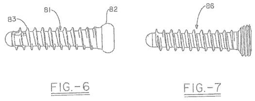
Figure 6 illustrates screw 81 with head 82 that is devoid of threads, and Figure 7 illustrates "locking" screw 86 with a head that has threads. *Id.* at 8:55–9:3. Screw holes 24 in plate 10 "preferably . . . can include internal threads which mate with external threads on the head of the screws to cause locking of the screws relative to the plate." *Id.* at 4:32–36.
