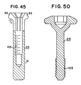
Figure 45 is a sectional view of buttress pin shank 23, and Figure 50 is a sectional view of pin head 25. *Id.* at 4:5–23, 8:63–67. In use, pin shank 23 is inserted into hole 57 or 63 of plate 13, until the flange of collar 93 is caught
