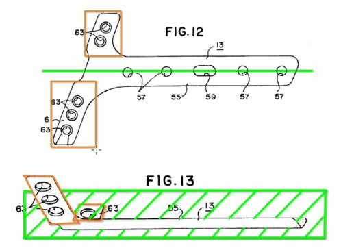
As set forth at pages 58–59 and 62–63 of the Petition, these annotations to Figures 12 and 13 of Grusin reflect how Grusin's plate 13 has an elongate central trunk portion having a medial longitudinal plane and
