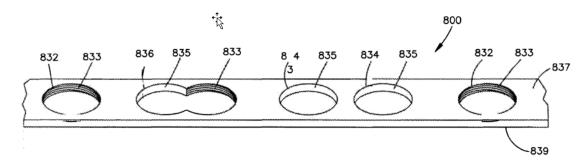
As described in Chan, Figure 8 illustrates bone plate 800 having "locking" holes 832 with threads 833 for engaging threads around the head of a locking bone screw, "non-locking" holes 834 with non-threaded or smooth inner surfaces 835, and "combination locking / non-locking" hole 836.
