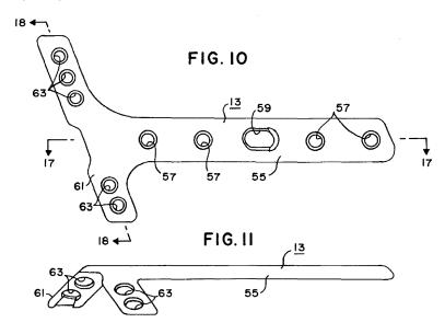
Figures 10 and 11 show, respectively, a top view and a side view of bone plate 13. *Id.* at 2:60–65, 6:60–64. Several spherically recessed holes 57 and 63 may accept either bone screws 37 as shown in Figure 76, or buttress pin shank 23 and head 25 combinations as shown in Figures 43–53. *Id.* at 5:66–6:1, 6:12–17, 6:60–7:6.
