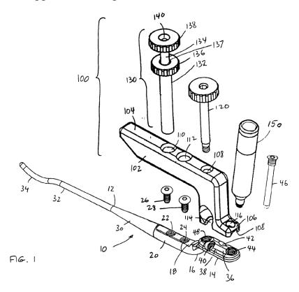
Figure 1 illustrates bone fracture fixation device 10 including threaded screw holes 22, 24 that receive the threaded shafts of cortical screws 26, 28. Ex. 1084, Fig. 1, ¶¶ 8, 42, 45; Ex. 1087 ¶ 27; Reply 5–6. The heads of screws 26, 28 are not threaded, so they are not locking screws. Ex. 1084, Fig. 1; Ex. 1087 ¶ 27. Thus, a person of ordinary skill in the art in
