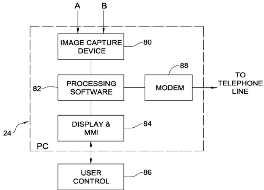
Figures 4A and 4B are block diagrams illustrating system 20 for confocal imaging of a 3D structure and providing a 3D monochrome entity.
