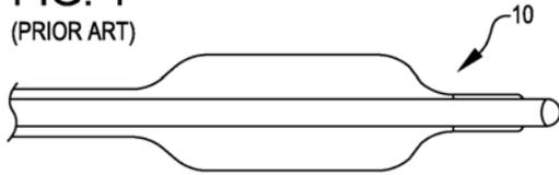
FIG. 1 is a view of the therapeutic end of a typical prior art over-the-wire angioplasty balloon catheter. *Id.* at 3:7–8.
