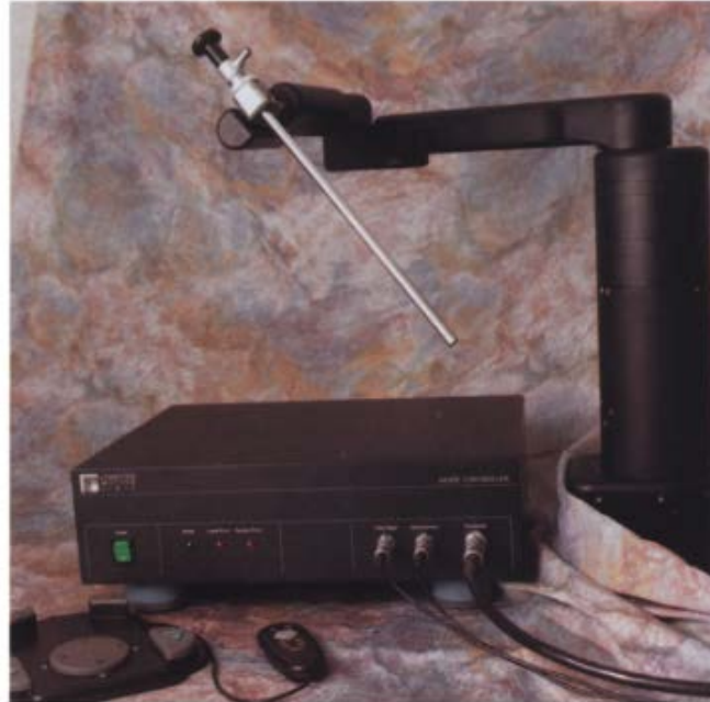
Fig. 1. A photograph of AESOP demonstrating the positioning arm holding the laparoscope, the computer control unit, the foot switch (bottom left) and the hand switch (bottom center)
