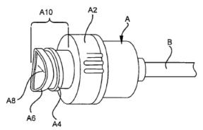
Ex. 1001, Fig. 1 (excerpted). As shown in partial Figure 1 above, "[a]ccess valve **A** includes housing **A2** with thread **A4** and septum **A6** with slit **A8**." *Id.* at 2:21–22.
