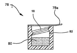
As shown in Figure 10B above, the "cap device" may include "threading **18** having a length that is less than inner circumference **82**." *Id.* at 5:31–32. The "cap device" may also include a "lid **78***a* and pad **80**." *Id.* at 5:16–17.
