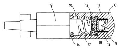
Figure 3 shown above is a "partially cut away side view showing the cover and port of the present invention after the cover has been tightly screwed over the port and the antiseptic capsule ruptured." *Id.* at 6:18–21.
