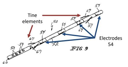
The Examiner stated that Borkan disclosed the claimed lead having a plurality of tine elements 67 proximal a plurality of electrodes 54 (Fig. 9 annotated above). Ex. 1002, 84-85. Since Borkan was silent on the use of an introducer, the Examiner relied on Memberg for use of an introducer, while Corbin taught
