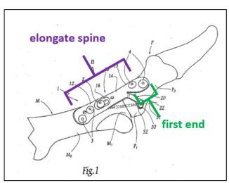
an arthrodesis plate "in the form of an elongated, generally flat body placed against the upper surfaces of the metatarsal and phalanx straddling the joint to be locked" having a first end (phalangeal portion 13) and a second end (metatarsal portion 12). (EX1008, ¶2, 14; Fig. 1).
