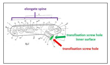
through the bridge portion (14) at a trajectory (longitudinal axis 31) configured to pass through a first position on the first discrete bone (phalanx P), a portion of the joint, and a second position on the second discrete bone (metatarsal M) once the plate is placed across the joint. (EX1002, ¶46, ¶¶258-260; EX1008, ¶¶6, 8, 23, 26-27, 32; claims 1, 3; Figs. 1-2, 5).
