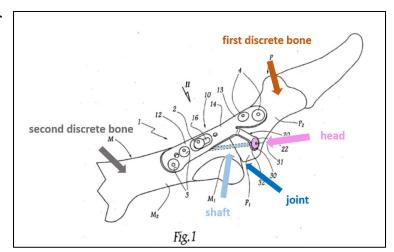
bone (metatarsal M in Fig. 1) so as to absorb tensile load when the second discrete bone (metatarsal M) is loaded relative to the first discrete bone (phalanx P) thereby transferring the tensile load from the second discrete bone (metatarsal M), through the screw (30) into said head (32) and said bridge portion (14). (EX1002, ¶¶261-262; EX1008, ¶¶6, 8-9, 26, 27, 32; claims 1, 3). As discussed above in Section VI.A.1.g., Slater also discloses this claim element.
