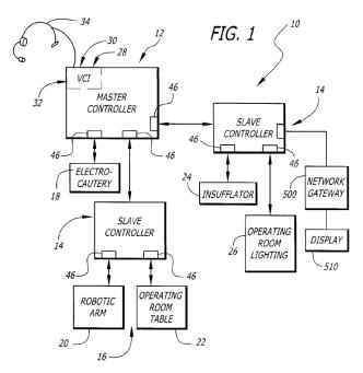
Figure 1 shows a block diagram of a general purpose master controller platform in electrical communication with slave controllers and operating room devices. *Id.* at 3:63–65. The general-purpose platform allows the doctor to manipulate the environment, and surroundings in order to keep movement in the operating room to a minimum. *Id.* at 4:49–5:4.
