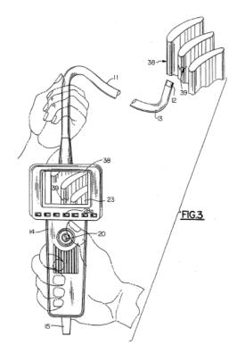
Figure 3 shows the handheld device with joystick that allows the operator to switch back and forth between steering the device and steering a cursor on a screen. *Id.* at 5:7–15.
