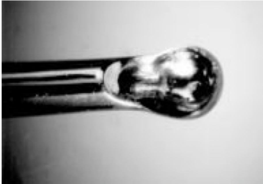
Figure 1 The tip of the ‘gonioscraper’. The bowl is 300 \mu m in diameter with its edges sharpened.
