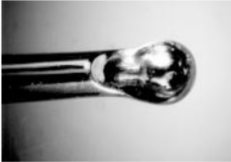
Figure 1 The tip of the 'gonioscraper'. The bowl is 300 \mu\text{m} in diameter with its edges sharpened.
