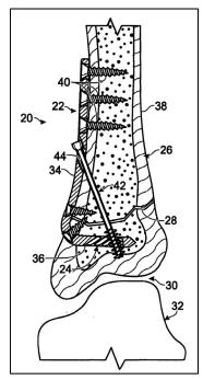
discloses that the "plate 22 may span a joint, such as joint 30 between tibia 26 and talus 32, among others." (EX1006, ¶21). The Falkner plate includes a first end (first plate portion 34) and a second end (second plate portion 36) secured to the bone(s) using bone screws that "may be placed into bone from any suitable number of openings of the bone plate." (EX1006, ¶¶23-24, 36-38). Threaded fastener 42 extends angularly through a bone fracture or a
