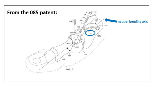
A POSITA would understand that "the neutral bending axis" of a given joint would fall approximately down the center of the adjacent bones, for each bone, depending on the cortical thickness on opposing surfaces. (EX1002, ¶152). In Slater, the axis of the bone plate approximates the direction of the neutral bending
