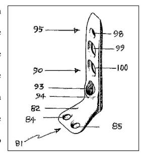
different points of the plate. (EX1005, 9:3-4). As can be seen at left, the unbroken portion of the plate that spans the ankle joint is thickened.
