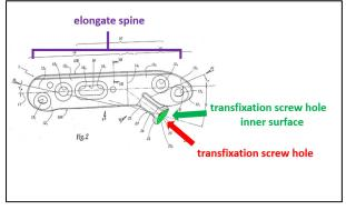
the transfixation screw hole (through-hole 25) such that the transfixation screw extends at a trajectory (longitudinal axis 31) configured to pass through a first position on the first discrete bone (phalanx P)and a second position on the second discrete bone (metatarsal M) once the plate is placed across the joint. (EX1002, ¶243-244; EX1008, ¶6, 8, 23, 26, 27, 32; claims 1, 3; Figs. 1, 2, 5).
