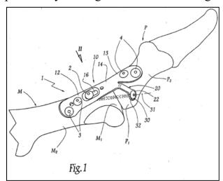
phalangeal part of the bone plate through which bone anchoring screws can be introduced into the metatarsal and the phalanx. (EX1008, Fig. 1). Arnauld further describes a leg of the plate that allows the plate to be attached to a dorsal-
