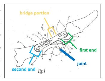
(EX1002,  $\P$ 241). For example, Arnauld explains that the "joint zone 14 between parts 12 and 13 is provided to overlie the joint zone between the facing epiphyseal ends  $M_1$  and  $P_1$  of the metatarsal M and phalanx P so that the plate body 10 straddles the metatarsal-phalangeal joint along direction 11." (EX1008,  $\P$ 14).
