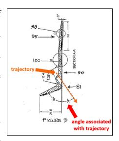
trajectory defined by the central axis of the inner surface of the transfixation hole crosses the neutral bending axis of the joint. (EX1002, ¶163).
