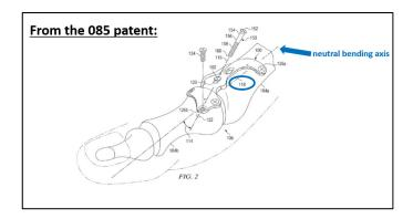
As shown in Figure 1, Arnauld discloses that the central axis 25<sub>1</sub> is configured to cross the neutral bending axis once the plate is placed across the metatarsophalangeal joint. (EX1002, ¶268; EX1008, ¶¶26, 27; Figs. 1, 4).
