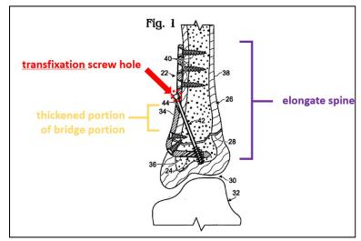
comprising an inner surface configured to direct a transfixation screw (threaded fastener 42) through the oblique opening 44 such that the transfixation screw 42 extends at a trajectory configured to pass through a first position on the first discrete
