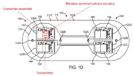
Pet. 25. Figure 1D of Libbus shows "printed circuit boards and electronic components over [Libbus's] adherent patch." Ex. 1004 ¶ 36. The electronic components shown in Figure 1D include "wireless communication circuitry 132." *Id.* ¶ 59. Petitioner has annotated Figure 1D to include a two
